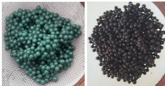
Figure 1: As-prepared HKUST-1 based microspheres (left) and MOF-74 (Co) based microspheres (right).
