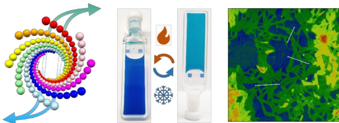
Figure 1. Molecular chains can be organized as supramolecular nanotubes that can be further tuned into metallogels for surface deposition purposes
